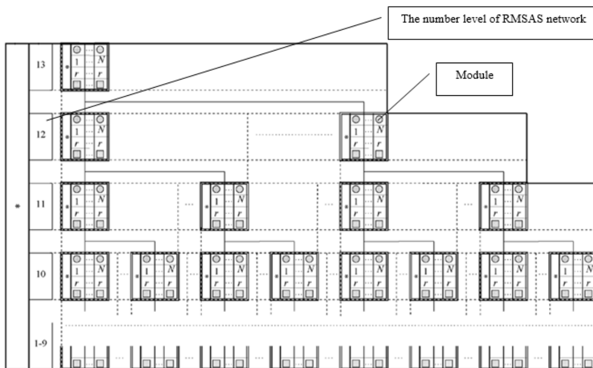
Fig. 2. Graphical representation of the reference model of the protected automation system (network) in the canonical form (Source: (Goldman R., 2002))
